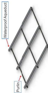
Installation node diagram (taking C-shaped steel purlins as an example)
