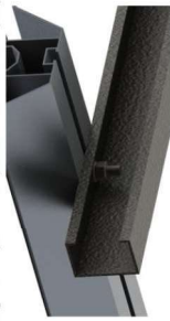
Installation node diagram (taking C-shaped steel purlins as an example)
