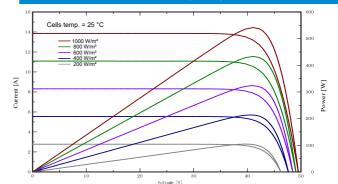
I-V Curve at Different Working Temperature (540W)
